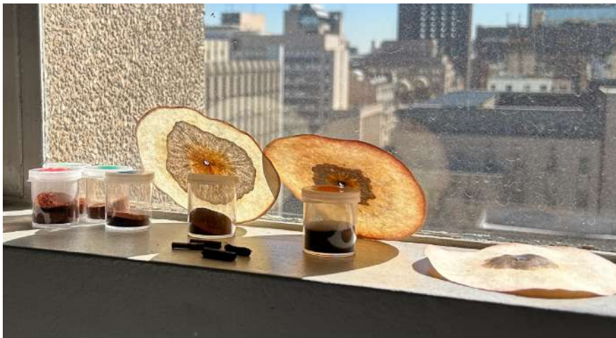
Figure 8. Chromatograms developing with the sunlight
